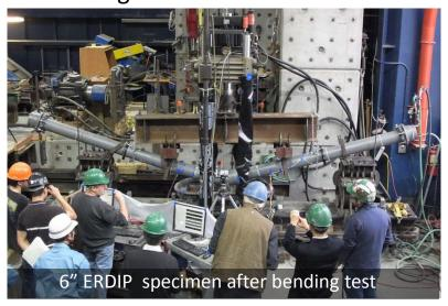
No leakage within the maximum deflection on 6", 12" and 16" ERDIP
